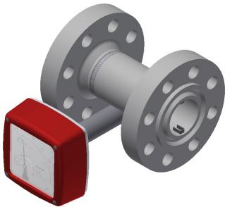
Through the unique structure of the measuring fitting with cylindrical measuring pipe and conical float, the units can be produced with thick walled pipes. This enables the use in high pressure applications for which other measuring instruments are not available e.g. sour gas, tunnel drill machine lubrication
