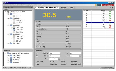
User interface of **iCom** (in the example: LEPTOSKOP 2042) with data administration for the gauge and PC, measuring parameters and list of readings. The top left window shows the file structure of the gauge. The currently selected file area of the PC hard disk is shown bottom left. By means of easy drag 'n drop you can copy the files of the gauge to the PC.
